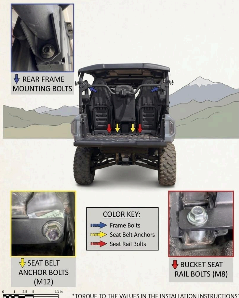
Bolt location diagram — Wolverine RMAX rear section.
